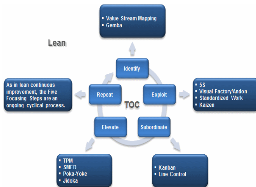
Figure 2. The display of the lean concept techniques by steps of the TOC Source: http://www.leanproduction.com/theory-of-constraints.html
